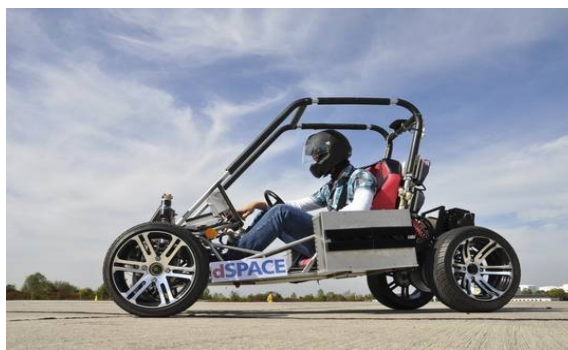
Figure1: electric vehicle based on a buggy chassis
