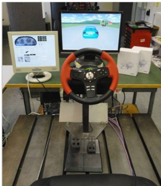
Figure 3: virtual test drive on the test bench
