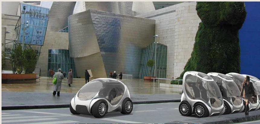
Launching in 2012. Price is estimated at 9.000€. It will be collapsible to facilitate parking, with a battery charging time of 12 minutes, 50 km/h of maximum speed and 120 km of range.
