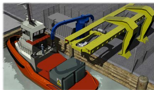
Figure 3-9: Series Hybrid-Electric Tug with Exchangeable Energy Storage (HET-EES)
