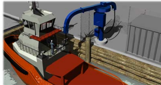
Figure 3-8: Series Hybrid-Electric Tug Concept with Plug-In Capabilities (HET-PI)
