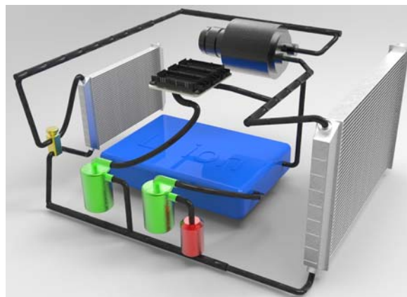
Figure 20. Total energy management system for an electric vehicle. The compressor (dark grey), evaporator, condenser and expansion valve (yellow) comprise the basic A/C system of the EV. The A/C system includes additionally two separate pumped cooling circuits, one for the power electronics (black) and one for the Li-ion battery (blue).
