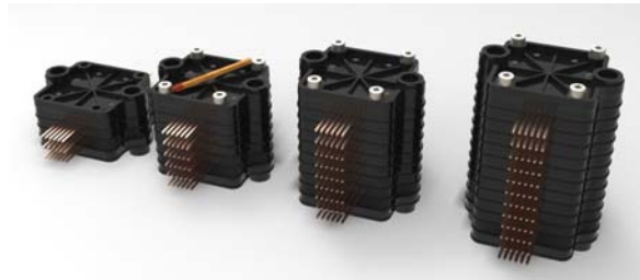
Figure 15. A family of stacked ShowerPower cooled transfer moulded power modules (Danfoss Silicon Power).
