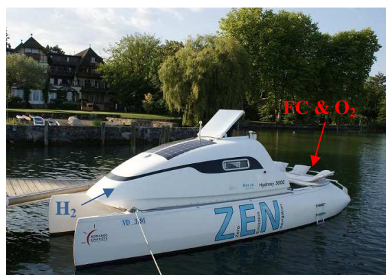
Figure 1: Catamaran with series hybrid FC/Battery power train propelled by 7 kW H 2 /O 2 fuel cell system.
