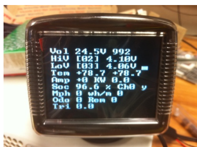
Figure 3: Master unit displays battery pack and cell voltage information
