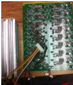
Figure 1: Secondary boards monitor up to 16 cells each
