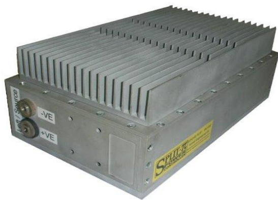
Figure 2 Current 4.5 kW Split-Pi controller as used in Green Power applications
