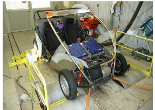
Figure 6 – Vehicle in test on ENEA rolling test-bench
