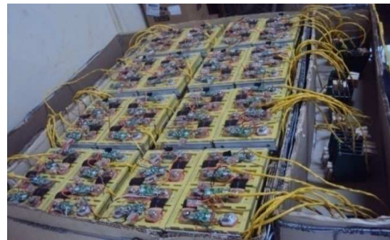
Figure 2: The Li-ion battery pack assembled
