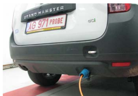
Figure 10: The traction battery recharging by coupling the GRAND HAMSTER E4WD to the Grid (220V AC/16A)
