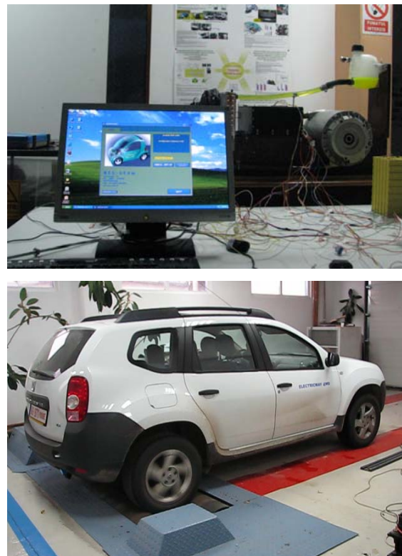
Figure 7: The Electric Drive System calibration with MES Software on the electric motor test bench (top) and on the vehicle roller test bench (down)
