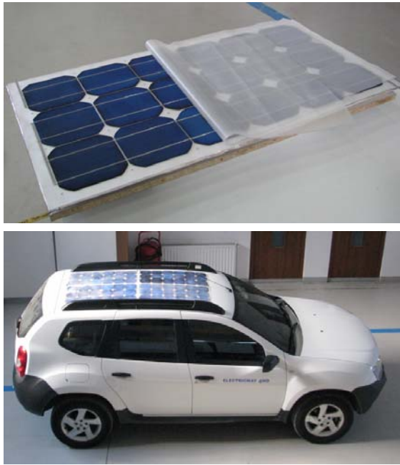
Figure 11: The photovoltaic module in construction (top) and the solar panel on the roof of the hybrid concept GRAND HAMSTER (down)
