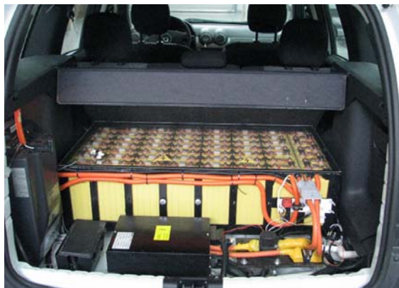
Figure 8. The traction battery (front) the Traction Inverter Module (back) and the on-board charger (left) placed in the rear side
