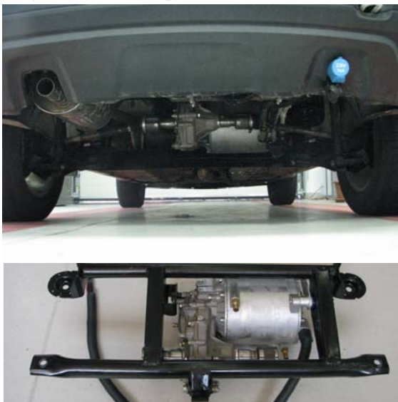
Figure 5: The rear axle and the electric drive mounted on the frame in the rear side of the GRAND HAMSTER E 4WD
