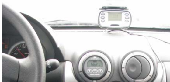
Figure 9: The traction battery monitor (205V) and the auxiliary battery (12V) monitor (down) and the VBox instruments (up).
