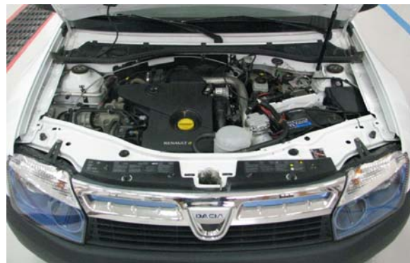
Figure 3: The engine compartment with the auxiliary new components: the electric vacuum pump and the electric motor throttle box.
