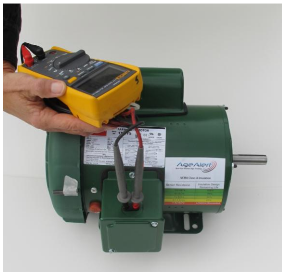
Figure 8: A conversion chart on the motor converts sensor resistance to percent remaining design life of the insulation based on actual motor environment and operating history. Alternatively, the sensor connects to wired or wireless condition monitoring systems.
