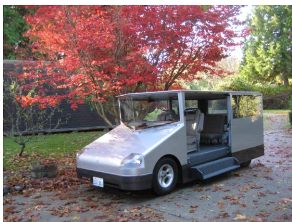
Figure 2: Ridek III modular vehicle with powered steps and sliding door to maximize user friendliness
