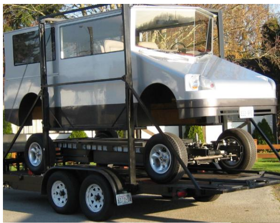
Figure 1: Modular vehicle with body lifted off
