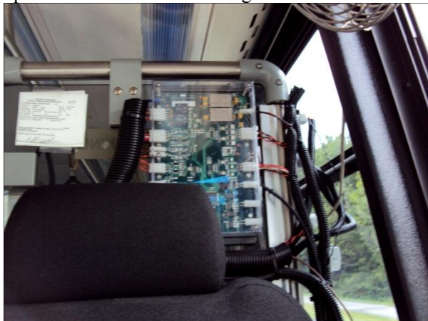
Figure 7 Battery Management System Control Board Mounted behind the Operator's seat
