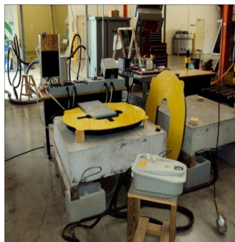
Figure 5 Stationary Coils, Pick-Up Coils (yellow) and Rectifiers in Background (covers off)
