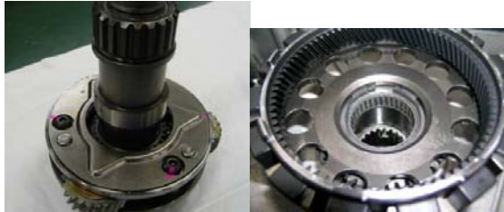
Figure 5 Planetary gear set (carrier/left, ring/right)
