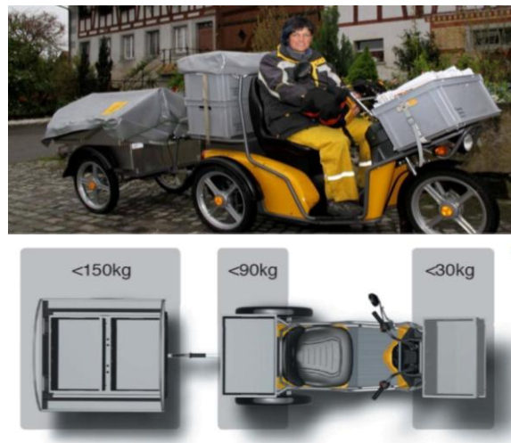
Figure 5: Kyburz DXP, a three wheel e-scooter for goods delivery
