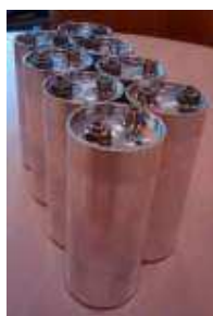
Figure 1: CEA LFBP/G prototype cells designs & corresponding electrical characteristics
