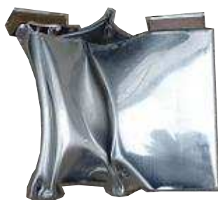
Fig. 8 Appearance of 20 Ah cell after the crush test in Y-axis.
