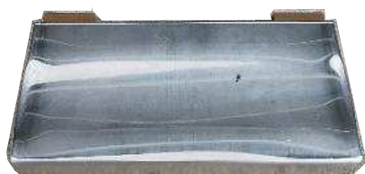
Fig. 7 Appearance of 20 Ah cell after the crush test in X-axis.
