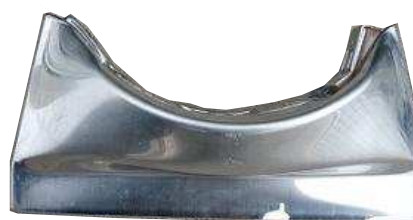
Fig. 9 Appearance of 20 Ah cell after the crush test in Z-axis.
