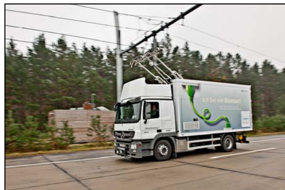
Figure 4 – Vehicle with current collector
