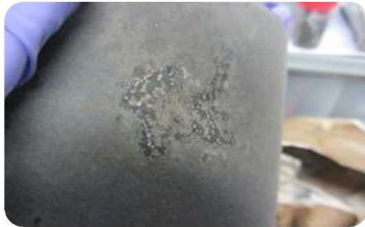
Deposit observed on negative electrode plate located near the edge
