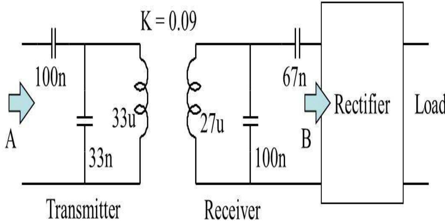
K. Throngnumchai et. al., *A Study on Receiver Circuit Topology of a Cordless Battery Charger for Electric Vehicles*, IEEE ECCE 2011, 843-850
