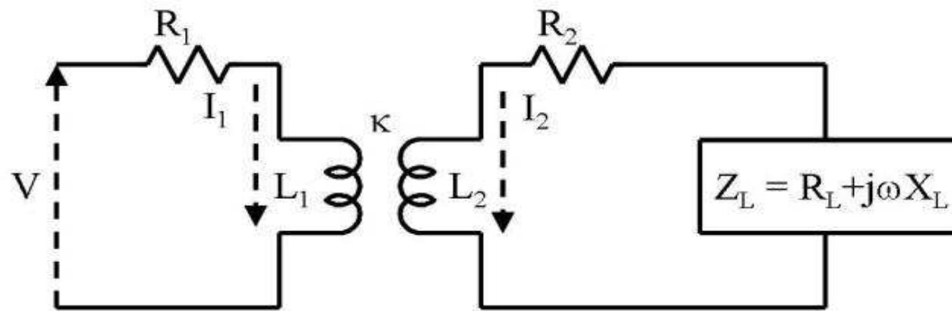
$$\eta = \frac{I_2^2 R_L}{I_1^2 R_1 + I_2^2 R_2 + I_2^2 R_L} = \frac{R_L}{\frac{(R_2 + R_L)^2 + (\omega L_2 + X_L)^2}{(\omega M)^2} R_1 + R_2 + R_L}$$
