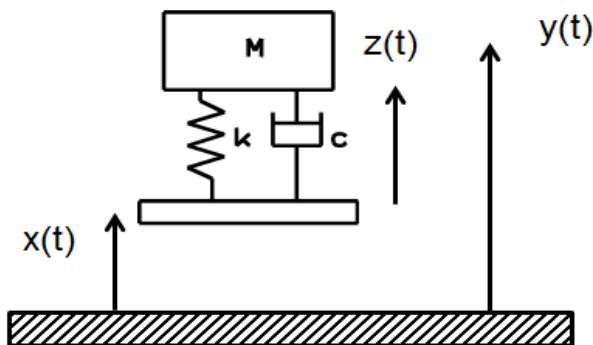
The simplest model of a dynamic system, the SDOF system (Single Degree of Freedom system)
