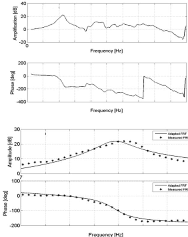
Dynamic response of a real system approximated with the response of a SDOF system
