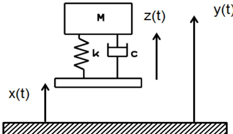
Instead of using the PSD, investigate the damage on SDOF models of the test object subjected to the vibration:
