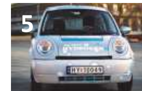
Retrofitted TH!NK with FC as range extender
