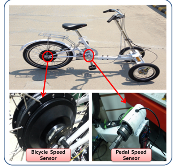
Figure 7: Pedal and Bicycle Speed Sensor Installation
