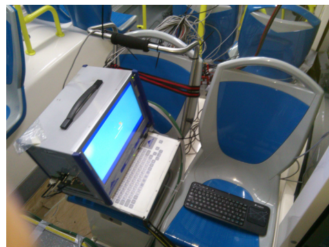
Figure 7: Measuring equipment employed in the full size hybrid urban bus tests.
