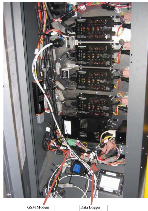
Figure 1: Typical Data Collection Installation on-board a city bus
