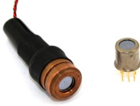
Figure 5: IR thermopile sensor with and without isothermal housing
