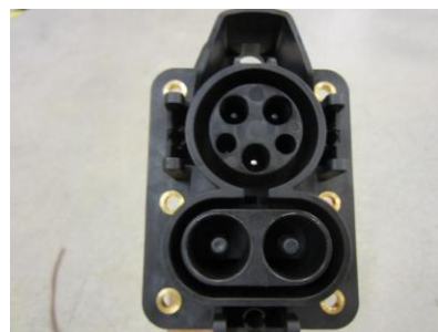
SAE Combo Vehicle Side Receptacle
