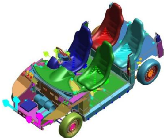
Figure 4: Discretised Microcab (FE) model (chassis)
