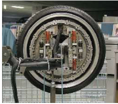
(c) Bridgestone's dynamic-damping in-wheel drive
