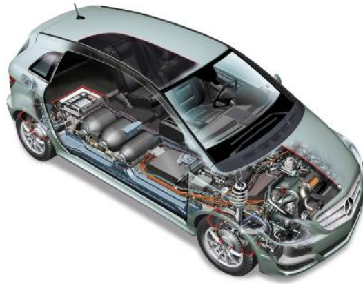
Figure 4. Schematic of the fuel cell system electric drive modules in the B-Class F-Cell. Source: Daimler AG
