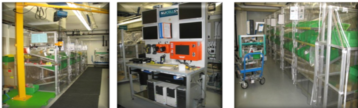
Figure 12. On the left side the production line of the air module, on the center the automated leak test and on the right side the assembly line of hydrogen module. Source: Daimler AG
