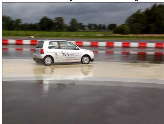
Figure 1: Understeering due to regenerative braking.
