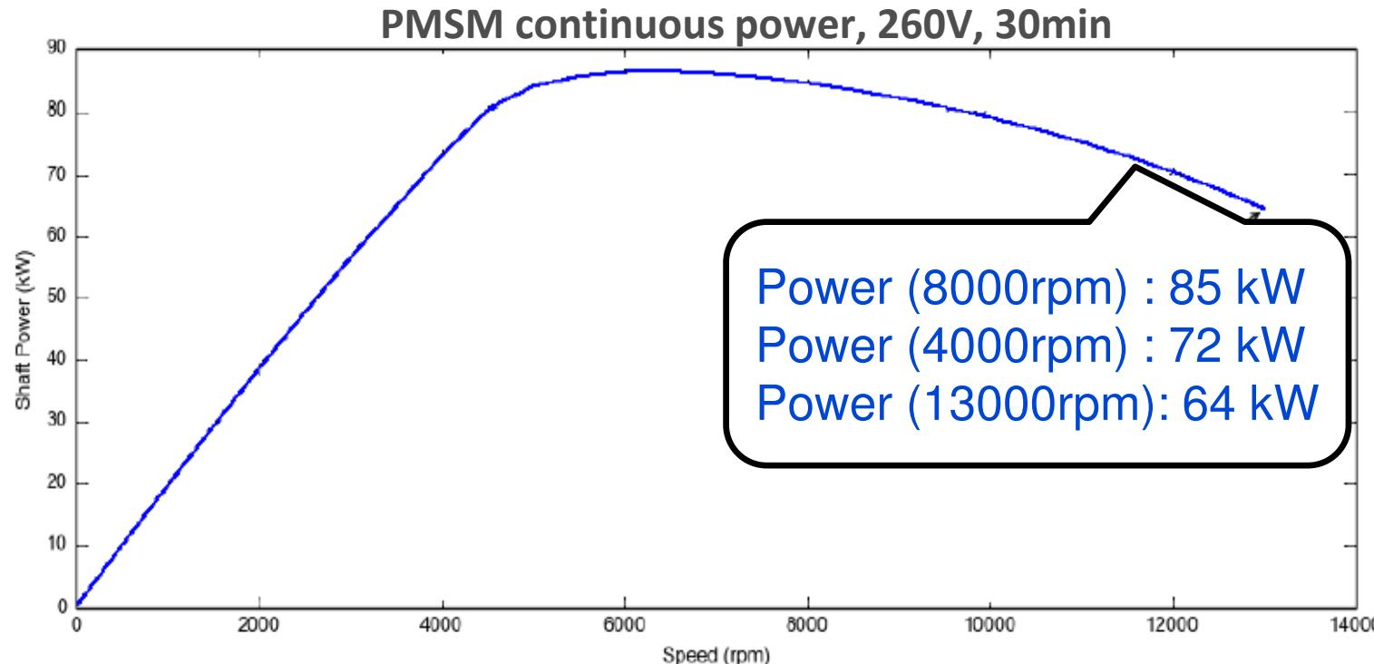
→ Limited by stator winding maximum temperature
