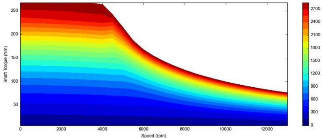
Rotor copper losses represents until 25% of the total losses  $\Leftrightarrow$  2,700 kW
