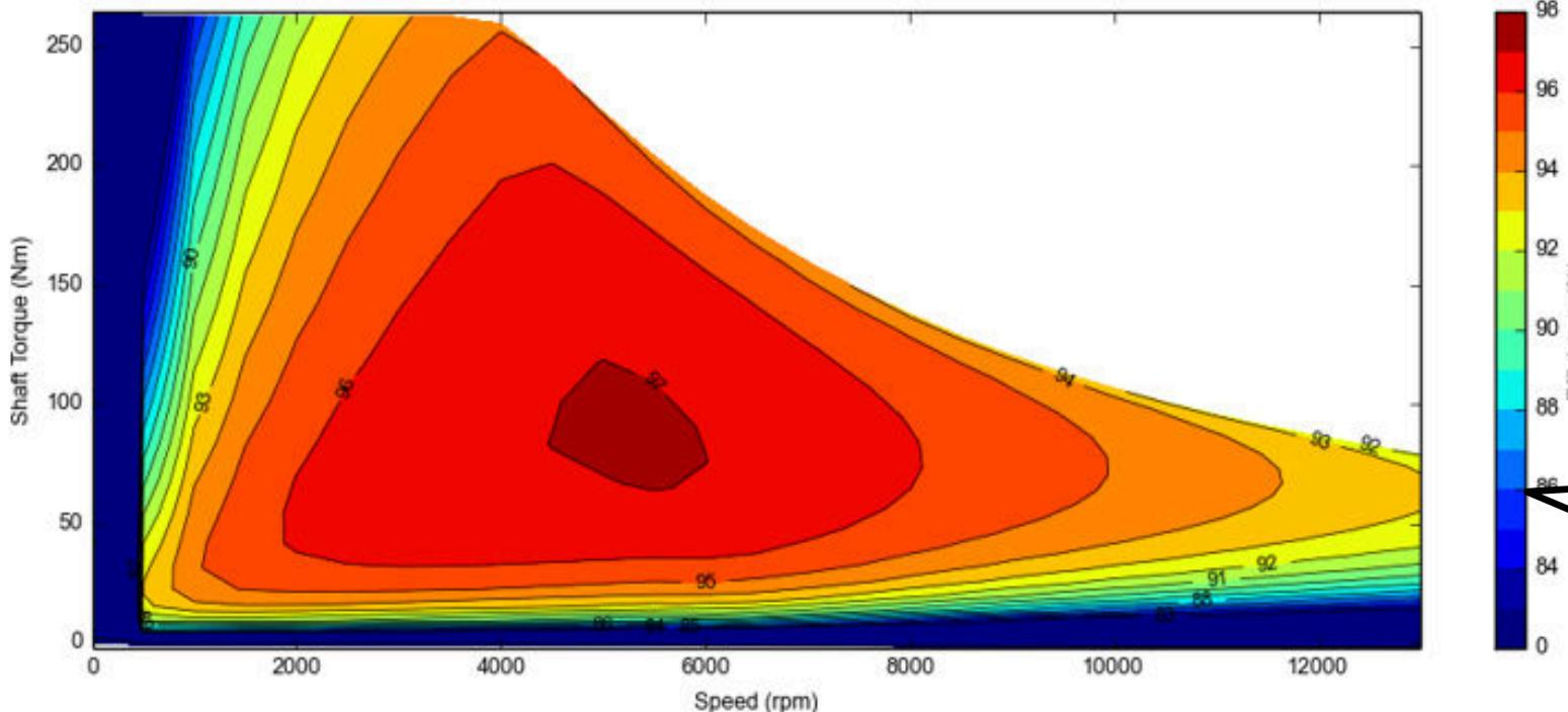
$\eta$  (5000rpm, 100Nm): 97,1%
