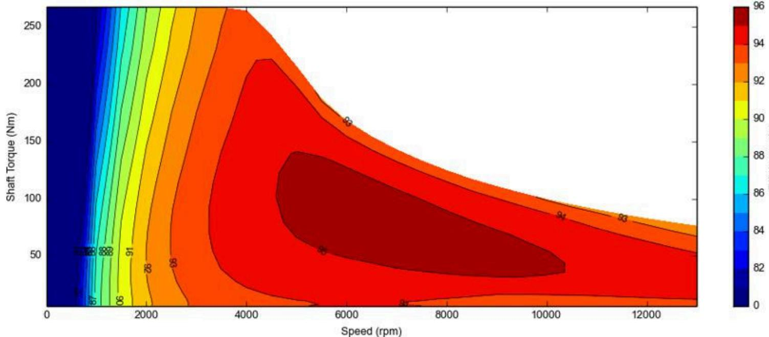
$\eta$  (6500rpm, 67.5Nm): 95,5%
