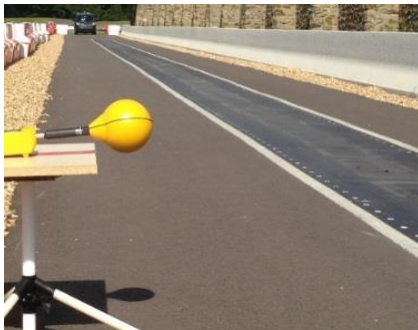
Figure 7(a): Experimental set up EMF emissions measurements
