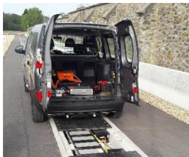
Figure 5(a): View of the first car prototype (the coils system and power electronics components embedded below the road covers can be seen)
