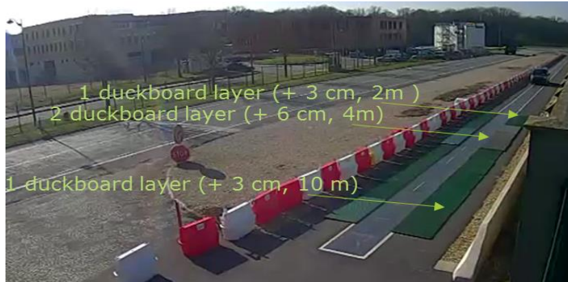
Figure 10: Two steps tests using different duckboard layers
