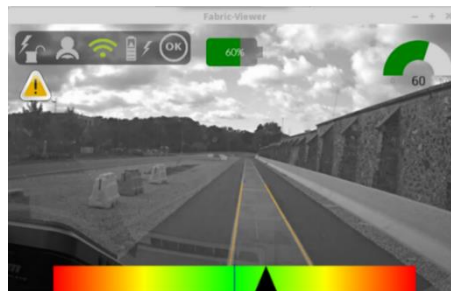
Figure 4: Alignment feed-back system integrated in the HMI developed for the FABRIC project
