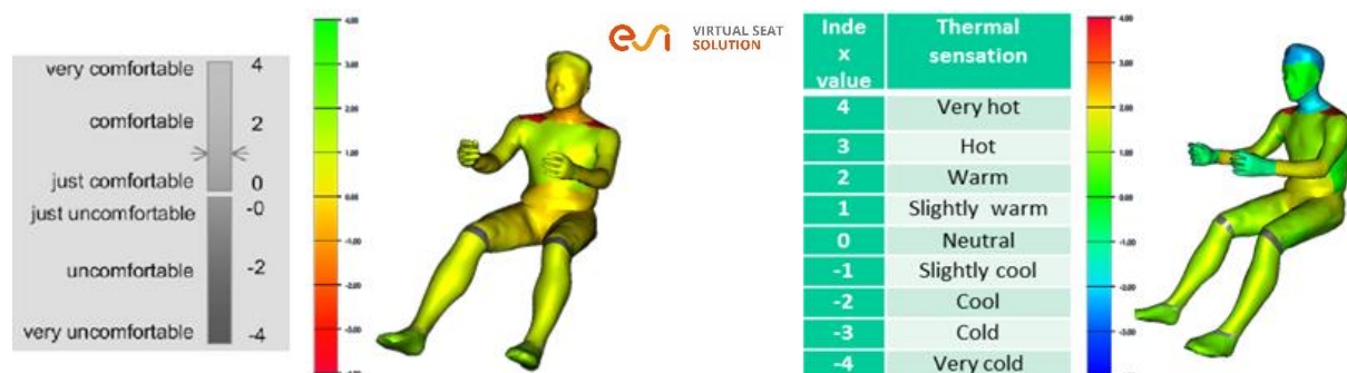
Figure 7: Thermal comfort and Thermal sensation indexes in ESI Virtual Seat Solution
