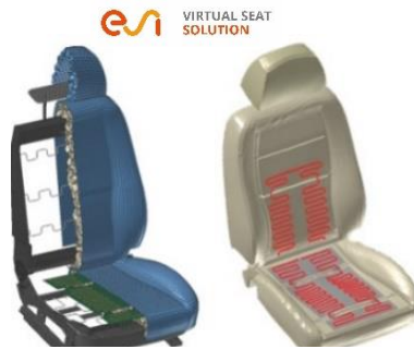
Figure 2: ESI's Virtual Seat Model with heating pad
