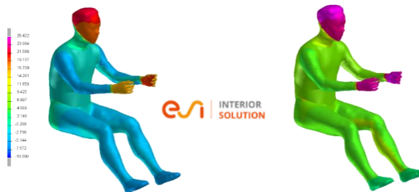
Figure 11: Temperature distribution on ESI human model (ESI Interior Solution) On the left the cabin temperature is imposed and constant, On the right, CFD is used for HVAC simulation
