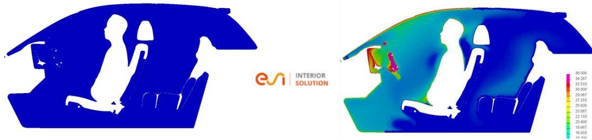
Figure 9: Temperature distribution results inside the cabin (ESI Interior Solution) On the left the cabin temperature is imposed and constant, On the right, CFD is used for HVAC simulation
