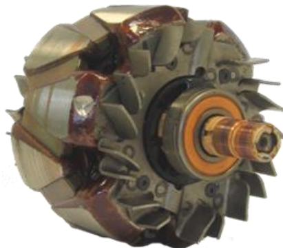
Figure 5: Alternator rotor and its claw shape poles
