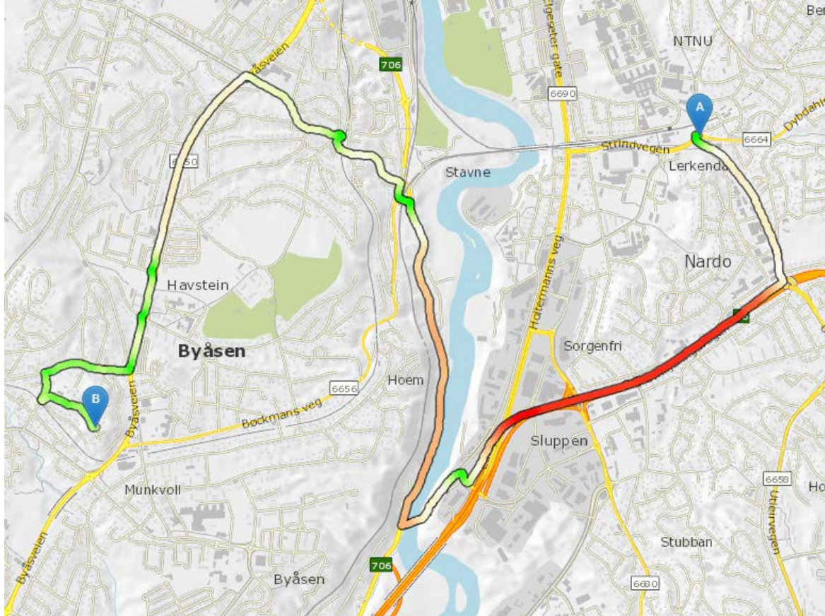
Figure 1: Speed estimation for a road transport route using a passenger vehicle. Red colour shows high speeds (70 km/h), obtained on the highway in this case, while green links shows lower speeds. Typically, steep hills, sharp turns and speed limits will influence the estimated speed for passenger vehicles.
