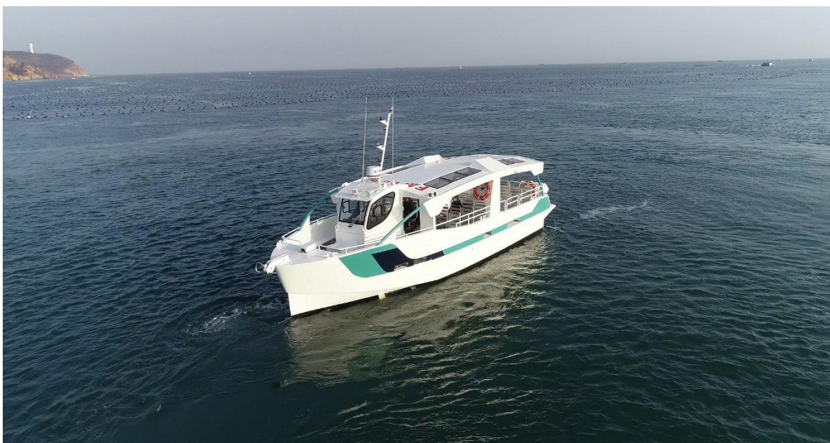
50 passengers plug in hybrid, Recyclable aluminum hull, Hybrid for clean navigation in protected areas, First diesels in France with Catalytic converter, Waterborne painting (Solvent free), LED and solar panels, Noise reduction...
