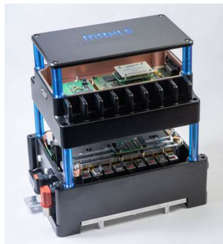
Figure 10: Exploded view of the battery pack, showing the individual sections (upper = BMS enclosure, lower = cell enclosure)
