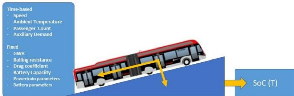
Figure 4 - Longitudinal Dynamic Model (BE-Bus), adapted from Towards ZEB transport, TNO
