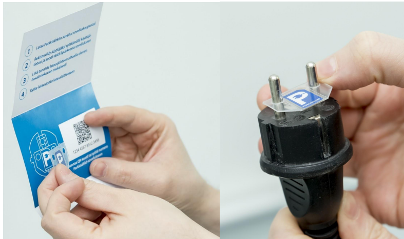
Figure 5: Parking Energy implements plug-and-charge in Schuko outlets by using an NFC ID installed in the Schuko plug. The Schuko socket has an NFC reader which detects the NFC for identification. The same technology is used for other traditional plugs and sockets.
