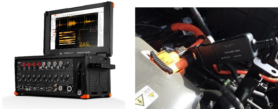
Figure 3. Measurement system R2DB Power Analyser (left) and mounted current clamp (right)
