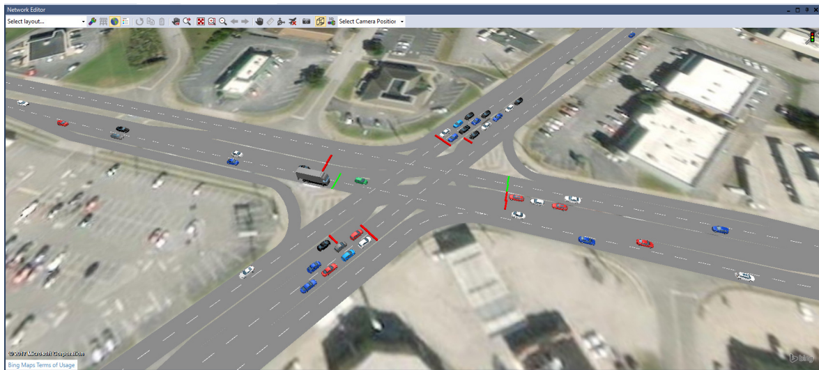
Figure 4: Traffic network developed and calibrated in VISSIM
