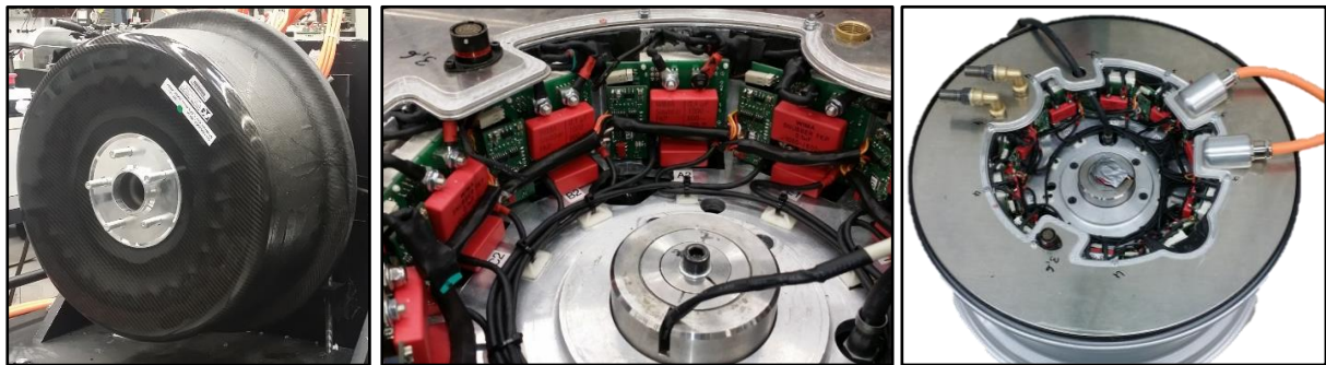
Figure 2: Back & front EVO 1 + integrated power electronics
