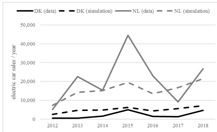
Figure 5: Model fit to historical Danish and Dutch sales data. Sources: data from [2] and own simulations
