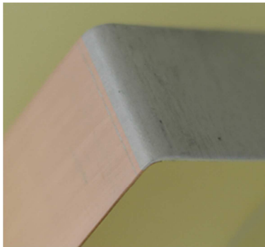
Figure 7: Specimens after tensile test (dimensions of specimen: 114 mm x 12,9 x 1,9 mm)
