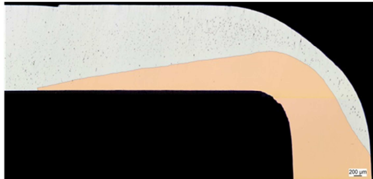
Figure 8: Specimen after 90°-bending test ( R = 1 mm)
