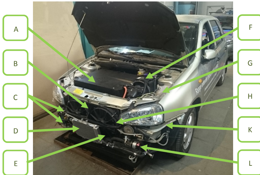
Figure 7: Electric vehicle with a Range Extender (A – high-voltage battery, B – primary radiator, C – electromechanical valve, D – radiator of the second circuit, E – electric motor, F – charger, G – expansion tank , H – inverter, K – pump 1, L – pump 2).
