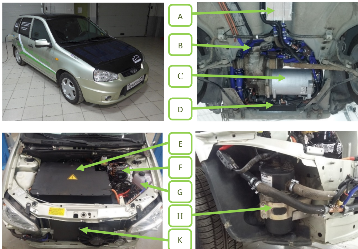
Figure 4: Electric vehicle equipped with the developed thermostating system (A – charger, B – pump, C – electric motor, D – inverter, E – high-voltage battery, F – cooler of liquid, G – expansion tank, H – electric heater of liquid, K – radiator with fan)
