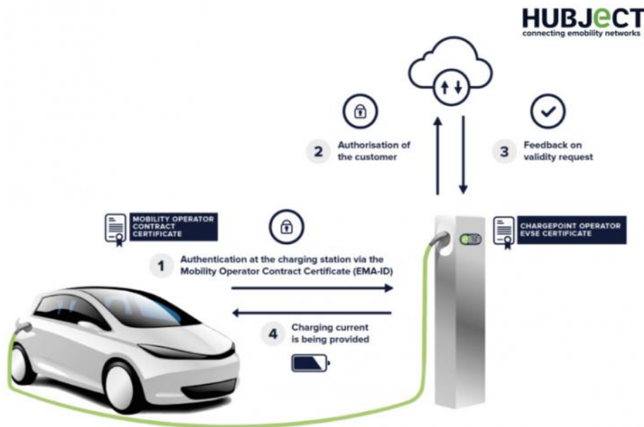
Figure 2 A high-level overview of the Plug and Charge certificate process [6]
