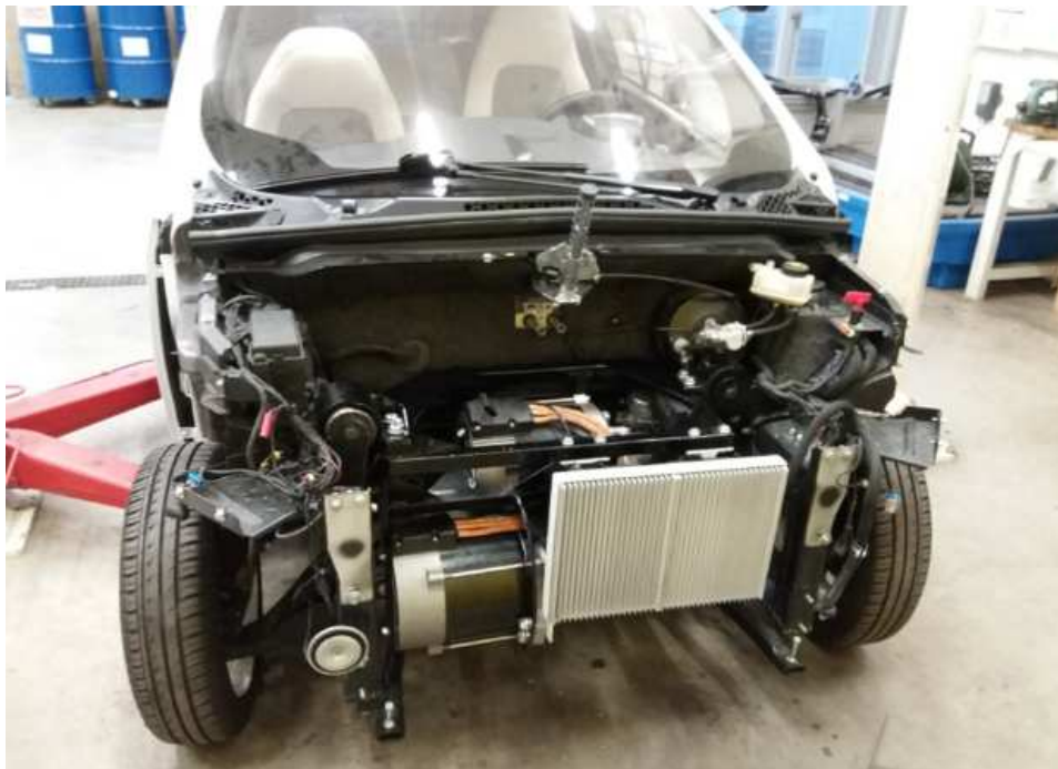
Figure 7: Photo of the eCULT's front with subframe and milled cooling devices for the inverters
