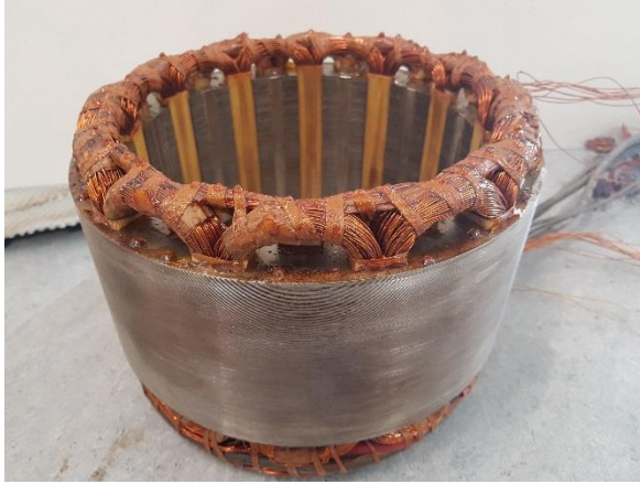
Fig.8(a): Wounded stator of HEFSMP
