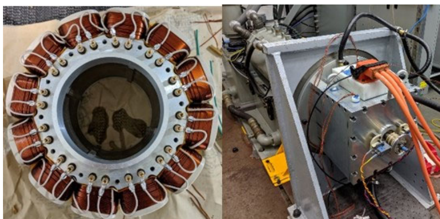
Figure 9: Square WFSM rotor (left) and overall WFSM rotor with brushes and slip rings mounted on the dynamometer for testing (right) (Source: Illinois Institute of Technology).
